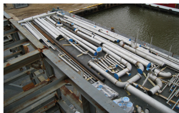
Stainless pipe spools loaded on barge for bulk shipment.
